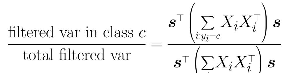
The CSP objective's outlier-sensitivity (see figure below) leads to the problem of overfitting.
